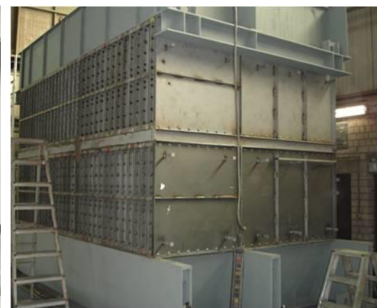
Module of a cast iron gilled plate heat exchanger
