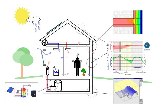
Hygrothermal models (e.g. WUFI® Plus) include all heat and moisture exchange processes between the interior spaces and the building envelope, furniture, etc.
