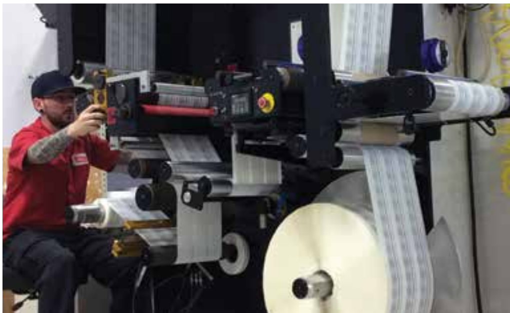
Self-adhesive labels in the slitting process
