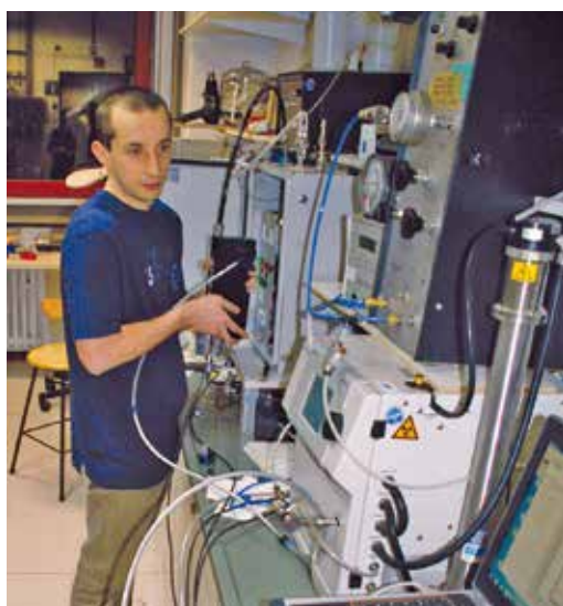
A JMSC PhD Student is analyzing the sizes of particles with a white light optical spectrometer
