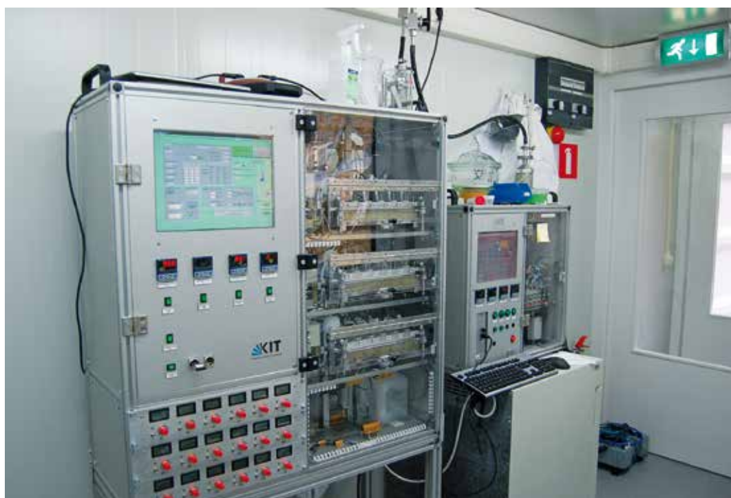
The Air-Liquid Interface (ALI) system in which the cells are exposed to emissions is constantly improved for the needs of HICE
