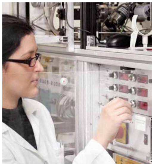
PhD student working on the photo ionization-mass spectrometer at the Chair of Analytical Chemistry in Rostock
