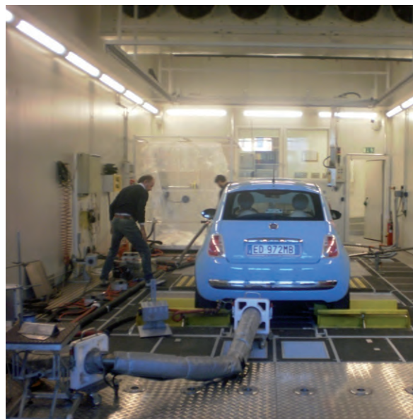
VELA experimental facility for Light Duty vehicles and mobile smog chamber from PSI during 2011 campaign in Ispra (Italy).
