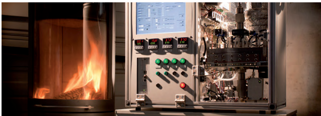
Compact Karlsruhe Exposure System used to assess the toxicity of nanoparticles and pollutants from biomass combustion. Image source: KIT.
