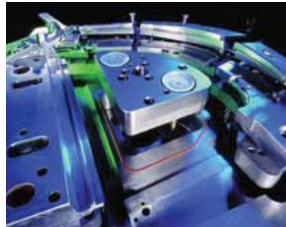
Complex glass encapsulation mold with multiple slides
