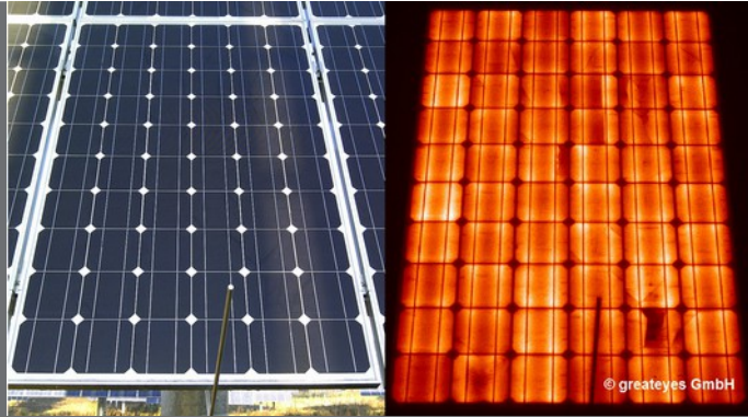
Inspection of single modules with battery-powered system
