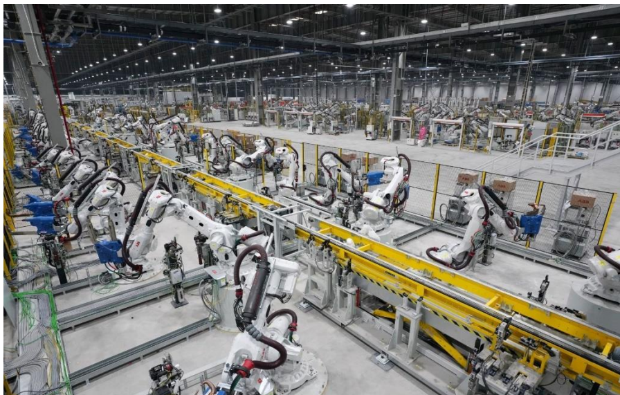
Figure 5: VinFast's factory with a complete welding solutions package from ABB (Photo: VinGroup)
