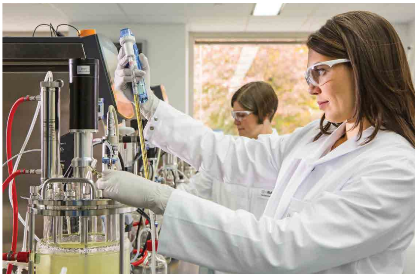
Research Scientists Allison Guinta (front) and Lauren Junker (back) take samples to examine fermentation products. Bio-based chemicals are produced under controlled microbial fermentation conditions. Optimization of fermentation conditions is an important part of the ongoing research at BASF's white biotechnology research center in Tarrytown, New York.
