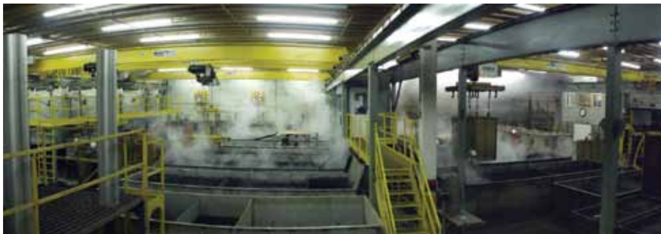
STEAG's catalyst regeneration plant offers two production lines for the refurbishment of power plant catalytic converters to provide significant cost savings to its customers and save precious resources.
