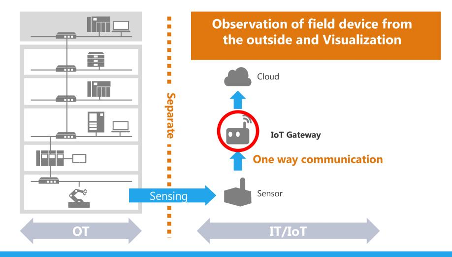
Separate OT and IoT It does not directly affect the control process
