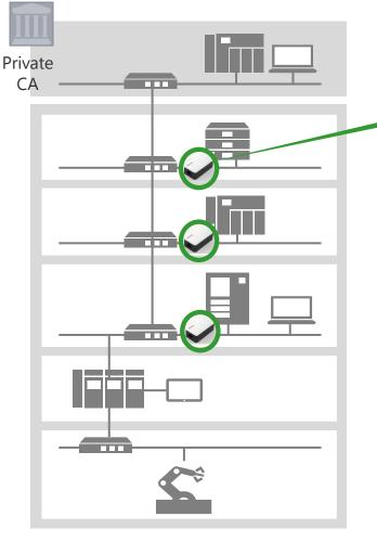
Secure security without changing existing system by inserting Secure Proxy Device just before endpoint legacy device
