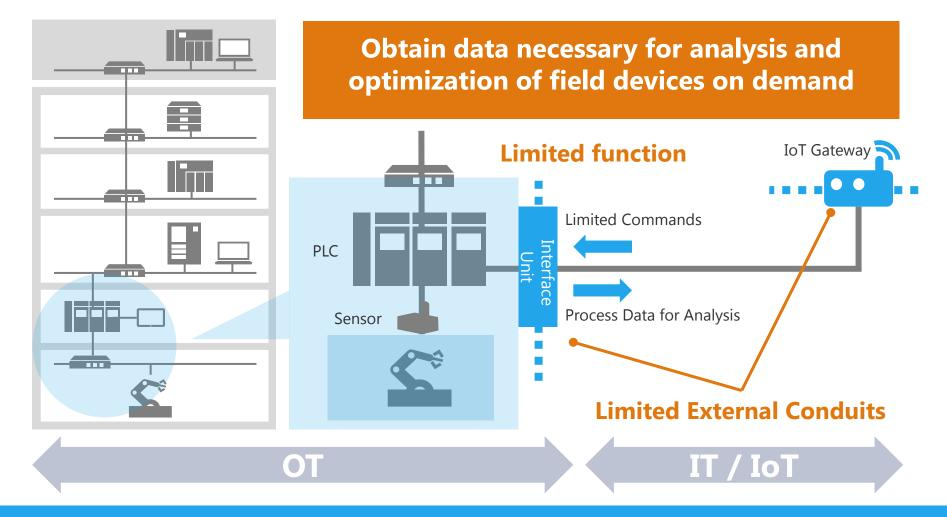
Limited external connections and functions It does not affect important functions of the control process
