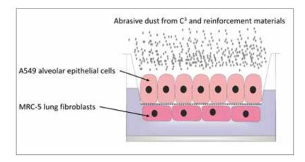
Figure 1: Schematic drawing of the cell culture model utilized to test the toxicity of the abrasive dust from C<sup>3</sup> material, thermally stressed C<sup>3</sup> material, and carbon rods reinforcement material. For the A549 monoculture, no MRC-5 lung fibroblasts were cultured on the basolateral side of the cell culture insert.
