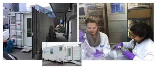
Figure 13: The HICE MobiLab, a mobile aerosol exposure and biosafety level 2 laboratory based on a 20 ft. shipping container. The HICE MobiLab contains two rooms. Left) HICE MobiLab in use at the University of Eastern Finland during a measurement campaign, the small insert shows the HICE MobiLab in Munich before shipping. Right) Photo of cell extraction and biological analysis work after cell exposures to wood combustion exhaust, taken through the HICE MobiLab window.
