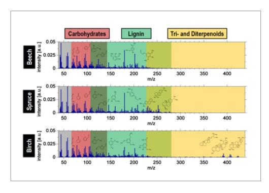
Figure 1: Mass spectra generated by thermal desorption of PM from the combustion of beech, spruce and birch wood with subsequent detection by single-photon ionization-TOFMS. Carbohydrates from cellulose pyrolysis and phenolic species from lignin decomposition are visible. A distinctive feature is the appearance of terpenoids with birch PM.
