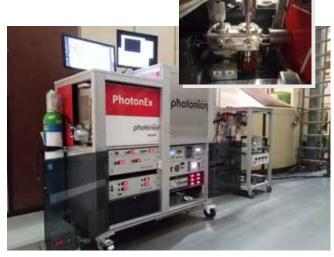
Figure 7: On-line gas-phase characterization. Dual on-line photoionization mass spectrometer (PhotoTOF; Photonion GmbH, Schwerin, Germany) for parallel acquisition of single-photon ionization using a VUV-lamp and resonance-enhanced multi-photon ionization (REMPI) mass spectra on a field campaign at the research laboratories of PROBAT-Werke von Gimborn Maschinenfabrik GmbH in Emmerich am Rhein.
