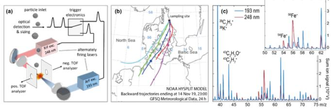
Figure 3: Setup for direct comparison of non-resonant and resonant ionization of Fe in ambient air particles using the same mass spectrometer. (b) Back trajectories ending at the sampling site during the experiment on long-range transported particles. (c) Accumulated cation mass spectra (n=15000) show a Fe+-signal enhancement for resonant ionization (248nm, red) versus the non-resonant case (193nm, blue) (Passig et al., 2020).
