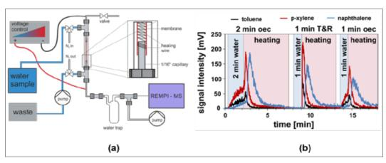
Figure 1: a) Experimental setup external hollow fiber membrane probe. b) Response behavior for toluene, p-xylene and naphthalene when applying the two variations of operation of the probe, open-end capillary or trap and release.
