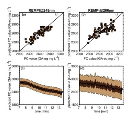
Figure 3: Top: Relation between measured and predicted FC value for REMPI at 248 nm (a) and 266 nm (b for calibration (dark brown) and external validation data set (light brown). Bottom: Model application on online data for FC value prediction in real-time with REMPI at 248 nm (c) and 266 nm (d) with predicted RMSEP (dark brown), prediction band (light brown), and measured FC value at drop of coffee beans (black cross).
