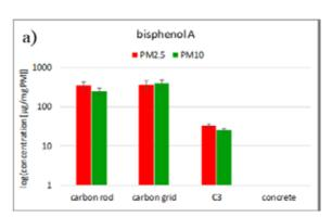
**Figure 1:** Bisphenol A concentrations in dust particles from the abrasive cutting of carbon concrete material. The reinforcement units (carbon rod and carbon grid) exhibit relative high concentrations, carbon concrete itself shows a lower content, concrete none at all.
