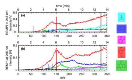
**Figure 2:** Combined mass spectra and time traces of individual roast gas components using REMPI at a) 248 nm and b) 266 nm. Grey-shaded area denotes the time-period referring to the displayed mass spectrum (reprinted with CC BY 4.0 License from Czech et al., 2020).
