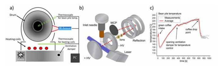
Figure 1: a) Coffee drum-roaster with a batch size of 100 g and thermocouples, b) setup of the laser based photoionization time-of-flight mass spectrometer and c) roast profile (reprinted with CC BY 4.0 License from Czech et al., 2020)
