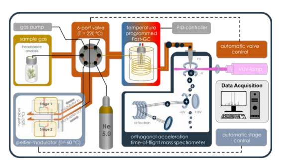
Figure 1: Schematic setup of the hyper-fast GC-SPI-TOF-MS system for headspace analysis of needles with sampling unit, 6-port-2way valve for changing to helium as GC carrier gas, Peltier modulator, optically heated fastGC, VUV-lamp for single-photon ionization (SPI) and oa-TOFMS.
