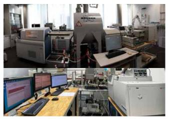
Figure 4: High-resolution MS laboratory in the Research Building LLM of the University of Rostock where the Chair of Analytical Chemistry/JMSC operates an FT-ICR MS System.
