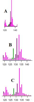
Figure 2: Small part of the naphthalene mass spectrum centered around the 128 m/z peak which is indicated in green on all 3 spectra, peak 128m/z is known to be naphthalene. Green shows the CH group, purple indicates the CHO group, and pink indicates the CxHyOz group with Z> 1.
