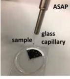
**Figure 1:** Photographic description of the particulate matter sampling from quartz-fiber filters for deploying to the atmospheric solid analysis probe. A tiny aliquot of the homogenously sampled aerosol is loaded to a pre-cleaned glass capillary and immediately transferred to the ASAP probe and into the ionization chamber, preventing contamination, at the same time starting data re-cording.
