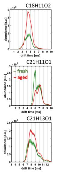
Figure 3: Selected drift time profiles based on species found in fresh (green) and aged (red) spruce emissions. Differences in the isomeric profile can be depicted. The shaded area is giving the standard deviation of three technical replicates.
