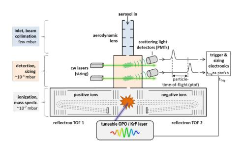
Figure 1: Working principle of SPMS: Particles are introduced into vacuum and optically detected and sized. In the current experiments on resonant ionization of metals, a tunable UV laser pulse is triggered when the particle enters the ion source of a mass spectrometer, producing positive and negative ions via resonant Laser Desorption/Ionization (LDI).
