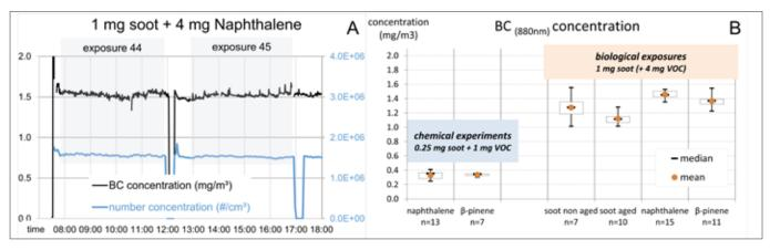
**Figure 3:** Short-term and overall reproducibility of seed particles production. A) Real-time data of black carbon and particle number concentration during two 4-hour exposure. B) Boxplot of BC concentration of all chemical experiments (0.25mg/m³ soot) and biological exposures (1mg/m³ soot).
