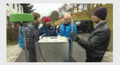
Measuring- and recording device for capturing particle matter of different sizes, particle number concentrations, aerosol particle size distribution, black and brown carbon.
