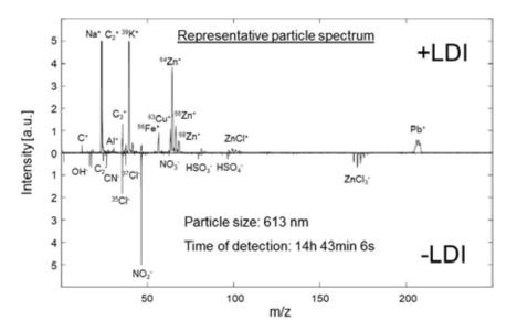
Figure 2: Representative +LDI and -LDI mass spectrum of particles of 4<sup>th</sup> July 2018 with significant loads of zinc, lead, iron, and copper.
