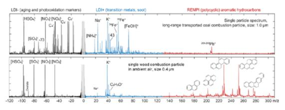
Figure 3: Exemplary mass spectra from two individual particles (top) If PAHs are absent, the technique yields bipolar mass spectra similar to conventional, LDI-based SPMS. (bottom) For PAH-containing particles, both inorganic ions, as well as a full-fledged PAH-spectrum is recorded, containing information on the particle's origin and aging processes during atmospheric transport (Schade et al., 2019).
