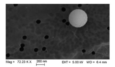
**Figure 1:** Scanning electronic microscopy (SEM) image of a fresh tarball particle generated from polar phase tarry solution. The morphology of the particles is perfectly spherical and amorphous in internal composition. Modified after Li et al., 2019.
