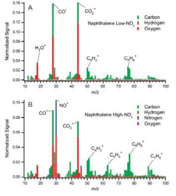
Figure 1: A and B are AMS mass spectra published in Chhabra et al., 2010. In A a result from a low NOx experiment is shown, 1B shows a result from a high NOx experiment, both at low precursor concentrations. Figure 1C shows a result of naphthalene aging from the aeroHEALTH campaign, with an equivalent aging of 2.4 days at 40% BH
