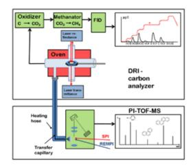
Figure 1: Thermal-optical carbon analyzer coupled to a photoionization time-of-flight mass spectrometer (TOCA-PIMS; reprinted with CC Attribution 3.0 License from Diab et al., 2015).
