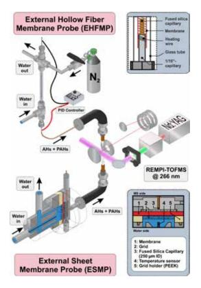
Figure 1: Overview of the developed membrane inlets for direct and fast analysis of aromatic hydrocarbons (AH) in water by resonance-enhanced multiphoton ionization (REMPI) coupled to time-of-flight mass spectrometry (TOFMS).
