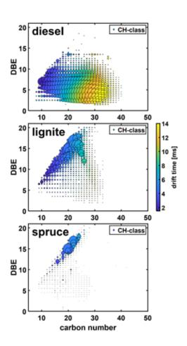
Figure 2: Molecular responses of the direct inlet probe approach given as carbon number versus DBE (CH-class) for the diesel, lignite, and spruce emissions. The apex peak position of the drift time (ion mobility response) is deployed for color-coding, whereas the size is coded according to the summed abundance of the respective elemental composition.
