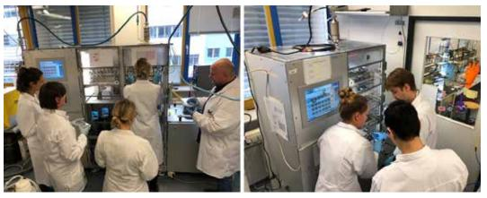
Figure 11: Bio laboratories at the CMA/JMSC location in Gmunder Straße in München Sendling. Three automated Air-Liquid-Interface (ALI) Exposure-Units are used to expose human lunge cells (cell lines and primary cells) to fine and nanoparticles and gases (aerosols) under realistic conditions to investigate the health effects of air pollution.
