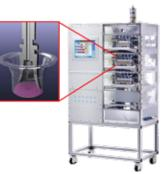
Figure 11: (left) The HICE-MobiLab during a measurement campaign for testing the biological activity and toxicity of shipping engine emissions (right) Mobile automated airliquid interface (ALI) exposure station for direct exposure of cell culture and co-culture tissue models to aerosols.
