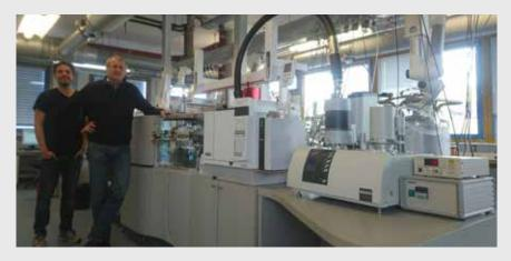
Prof. Zimmermann together with Dr. Uwe Käfer at the first LECO Pegasus HRT 4D System. The system is equipped with a direct insert probe, soft photoionization and a hyphenation for thermal analysis. Main applications will be the investigation of aerosols for the Helmholtz International Lab "aeroHEALTH".
