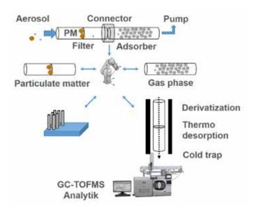
**Figure 1:** Concept for a simultaneous sampling and analysis of particulate and gas phase of (environmental) aerosols. Main components of the system will be a unit for sampling, desorption and chromatographic-mass spectrometric analysis.
