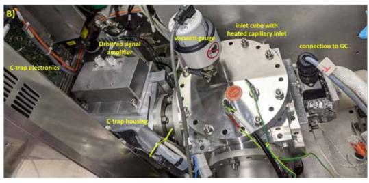
Figure 1: Scheme and photographs of the laser-based photoionization high-resolution mass spectrometer (RFMPI Orbitrap MS). A) View on the laser-system depicting the Nd:YAG solid-state laser (266 nm) and the inlet window into the C-tran housing. B) View on the sample inlet side showing the inlet cube with heated capillary, connection to the gas chromatograph (GC). and C-trap housing with attached Orbitrap analyzer
