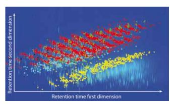
Figure 1: Preliminary measurements with comprehensive two-dimensional gas chromatography of the Ichthyol matrices reveals a very complex isomeric pattern of sulfur compound classes. The graphs show a part of a typical two-dimensional separation with focus on sulfur classes. Each dot represents an individual compound, those dots are grouped according to their chemical functionality. ( Thiophenes, Tetrahydrothiophenes, Dihydrothiophenes, Naptha-folefino-thiophenes, Benzothiophenes)
