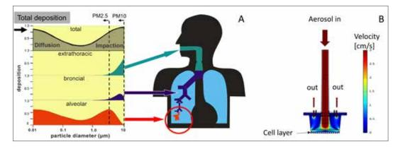
Figure 1: (A) Particle size dependent lung deposition - model results from the "Hygroscopic Particle Deposition Model" by Ferron et al. (HPLD06 online calculator, see https://www1.helmholtzmuenchen.de/ioec/lungdeposition/hpldb06\_d/ index3d.php, and report (14) in Research Area 1). (B) Calculated aerosol velocity profile of the "Air Liquid Interface" (ALI) exposure unit.
