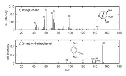
Figure 1: SPI mass spectra of a) levoglucosan and b) 3-methyl-4-nitrophenol.
