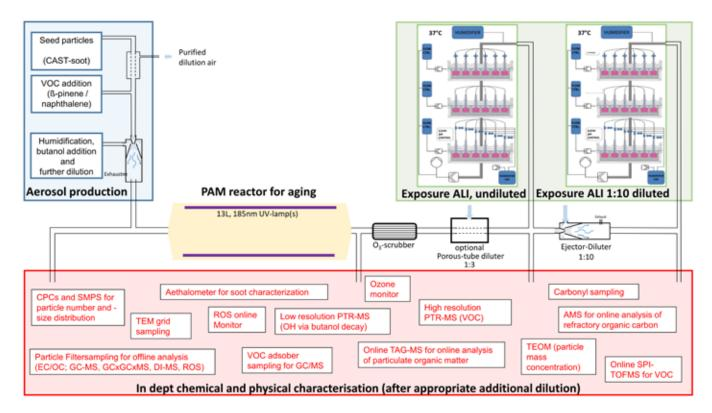
**Figure 2:** A simplified experimental scheme of the aerosol generation, aging and SOA formation (PAM), aerosol characterization (see also figure 1), and Air-Liquid-Interface (ALI) cell exposure setup (see reports aeroHEALTH 5-8 for more details).
