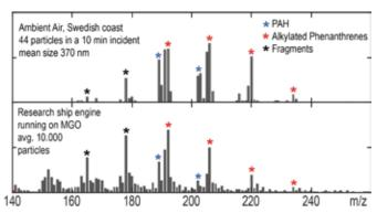
**Figure 4:** top: Mass spectra of aromatic molecules from a transient event in Sweden (17<sup>th</sup> Oct 19, 00:30). bottom: Mean particle spectra from the research ship engine in Rostock, running on Marine Gas Oil (MGO). Dominant signals of alkylated phenanthrenes in the respective m/z-region are indicative for MGO combustion on ships.
