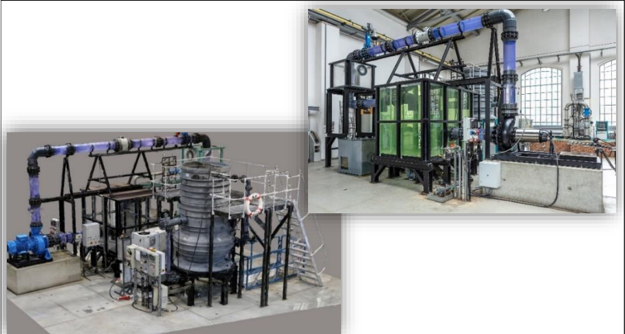
Caption: From the virtual to the real world: The digital representation of a demonstration model of a wastewater pump station at TU Berlin (L), with the real plant at right.
