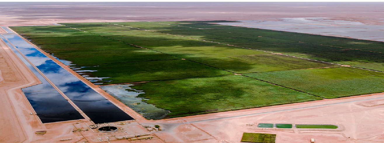
Nimr Water Treatment Plant: The world's largest constructed wetland developed by BAUER Resources GmbH in Oman to treat produced water from the oil & gas industry.
