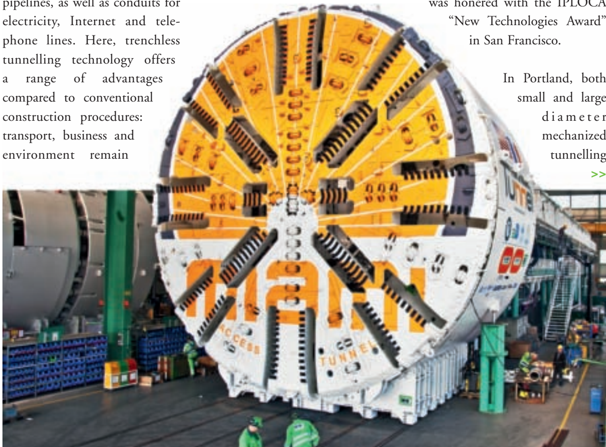
Workshop acceptance of the tunnel boring machine for the Miami Port Tunnel.
