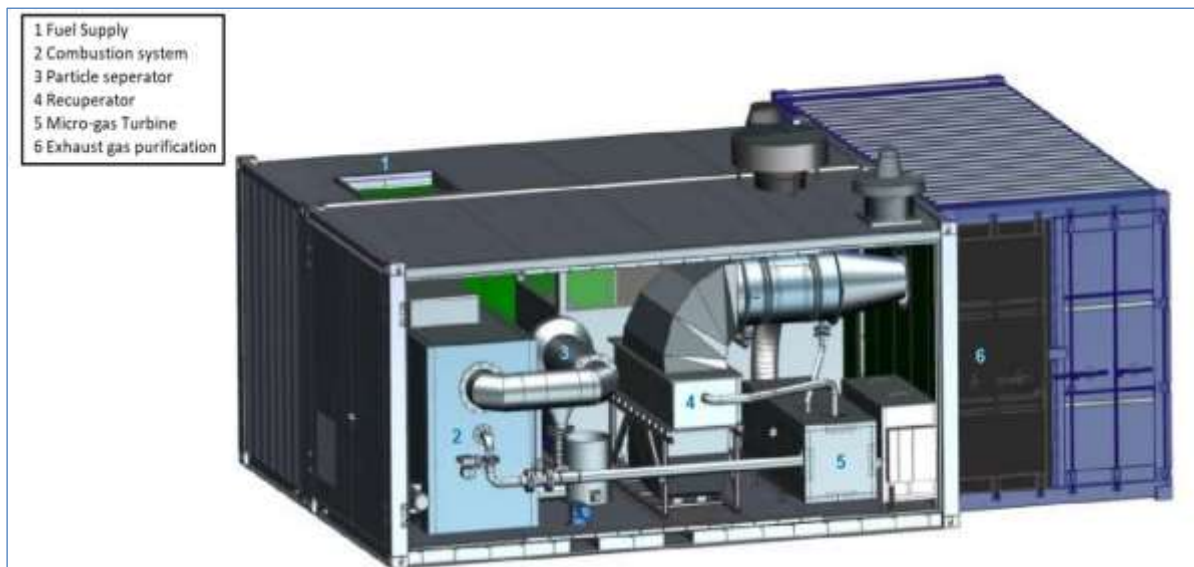
Figure 20: Budget-line 2: Additional externally fired gas turbine (EFGT), (Source: www.bergundkiessling.com )
