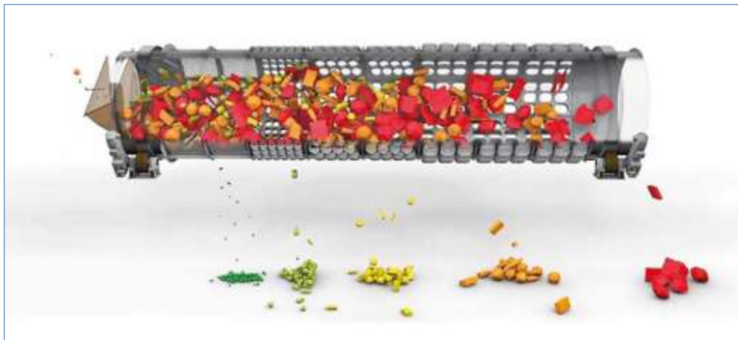
Figure 15: Example: trommel screen (Source: www.w-stadler.de )
