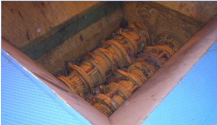
Figure 14: Example of an automated Bag opener (Source: www.coparm.net )
