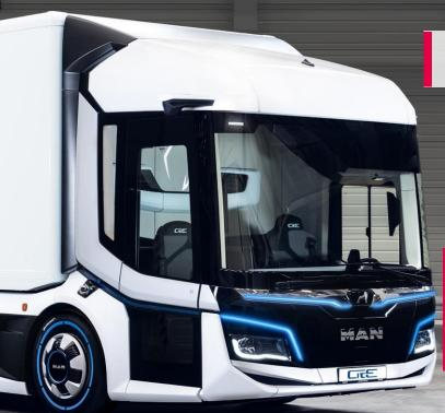
Ergonomic design with low access, continuous level driver cab floor and easy accessibility
