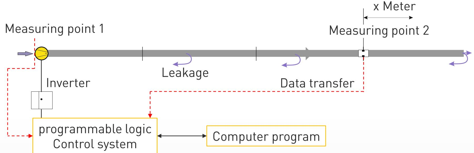
► system consists of a pre-determined fan, the duct, two measuring devices, a PLC, a frequency converter and a computer program
