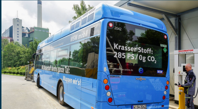
Turnkey project incl. 1,5MW Electrolyser and HRS for the H 2 infrastructure and refueling stations for up to 40 green-hydrogen powered buses in Wuppertal, Germany (2020).
