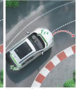
Oversteer T_{FA} < T_{RA}
