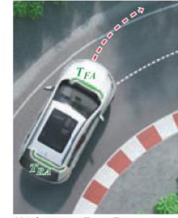
Understeer T_{FA} > T_{RA}
