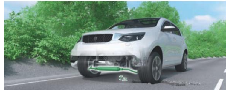
Decoupling: actuator torque front axle T_{FA} \approx 0
