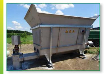
**Funnel systems** from 5 m<sup>3</sup> to 30 m<sup>3</sup>. These systems are entirely made from stainless steel and offer a feed power of 50 m<sup>3</sup>/h.
