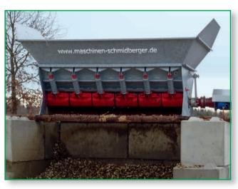
**Turnip shredders** of 1 m to 3 m size with an adjustable shredding power between 10 t/h and 20 t/h.
