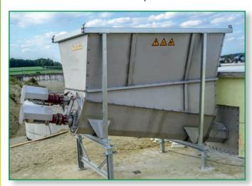
**Inclined inserters** from 3 m<sup>3</sup> to 30 m<sup>3</sup>, entirely made from stainless steel with a feed power of 50 m<sup>3</sup>/h. Optional covers are available. These machines are equipped with a 400 mm screw conveyor as standard.
