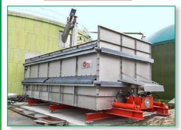
**Push floor dosing feeders** from 40 m³ to 120 m³. Made entirely from stainless steel, these machines offer a feed power of 50 m³/h. Weighing equipment and central lubrication are available. Can be made accessible for vehicles on request.
