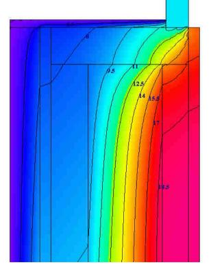
Analysis by simulation: Window frame & wall connection zone
