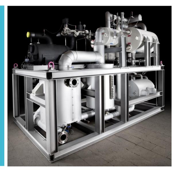
Cooling capacity: 280 Kw **Brine Cooling** Brine in/out: -3/-8°C Hot water in/out: 95/80°C Cooling water in/out: 25/30°C COP = 0.4 App: food superstore
