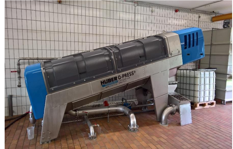
Sludge Dewatering with the HUBER Screw Press Q-PRESS®
