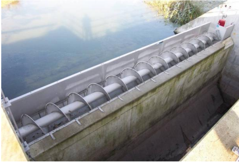
ROTAMAT® Storm Screen RoK 1 at an overflow
