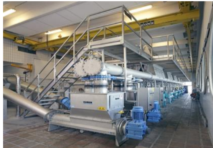
Screenings treatment with launder channel
