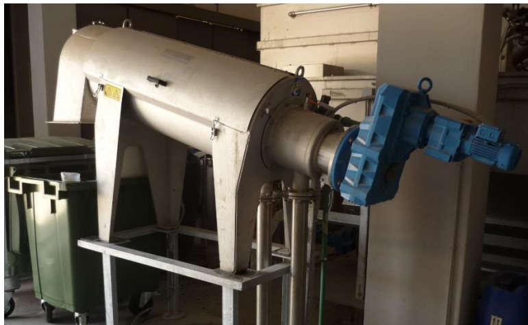
sludge dewatering with Q-PRESS WWTP Costa Navarino
