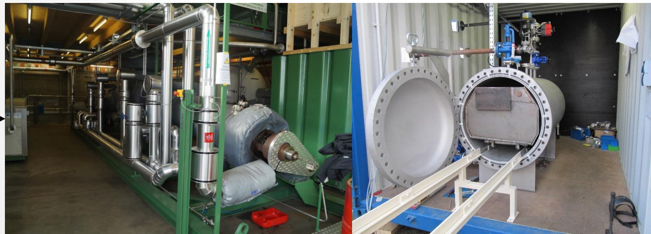
HTC-Reactor (< 30% DM) or VTC-Reactor (> 30% DM)
